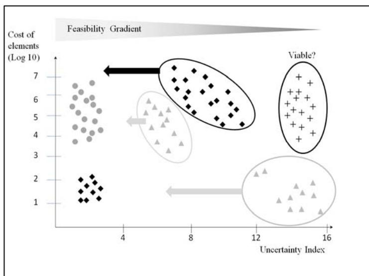
Figure 1: The concept as fully developed into a decision-support tool. For each considered element, an uncertainty index is calculated, based on the level of uncertainty (available knowledge on the costs) and the nature of the costs (behaviour of the costs) and mapped against element costs on a  $\log_{10}$  scale.
