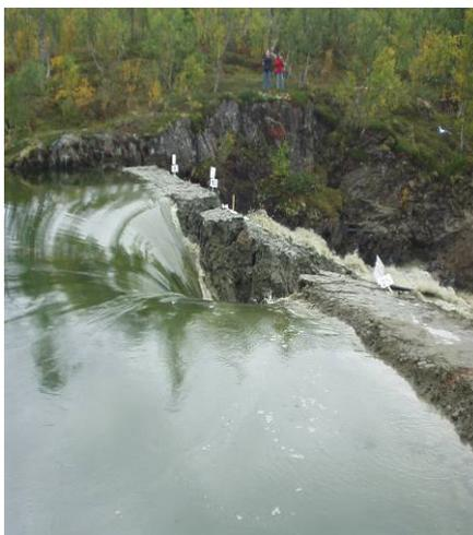
AREBA provides rapid prediction of the potential flood hydrograph for both overflow and internal erosion (piping) processes, assuming either surface or head cut erosion processes. The model also allows for the effects of surface grass cover. The model is applicable for simple homogeneous earth embankments. AREBA models the physics behind breaching in a simplified manner and:
