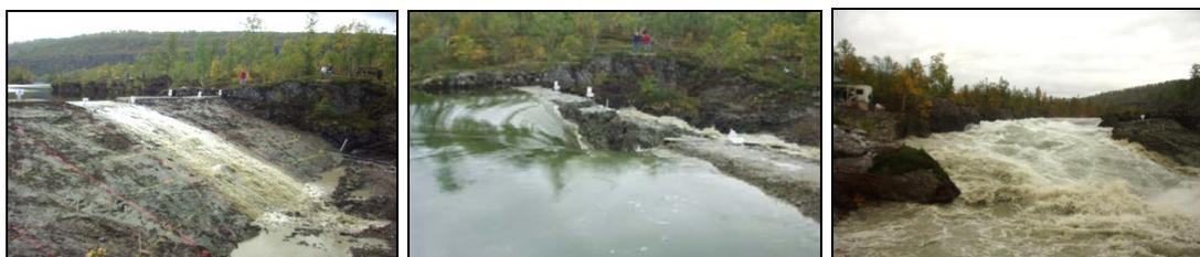
Figure 1: Three stages of breach flow (source EU IMPACT project)
